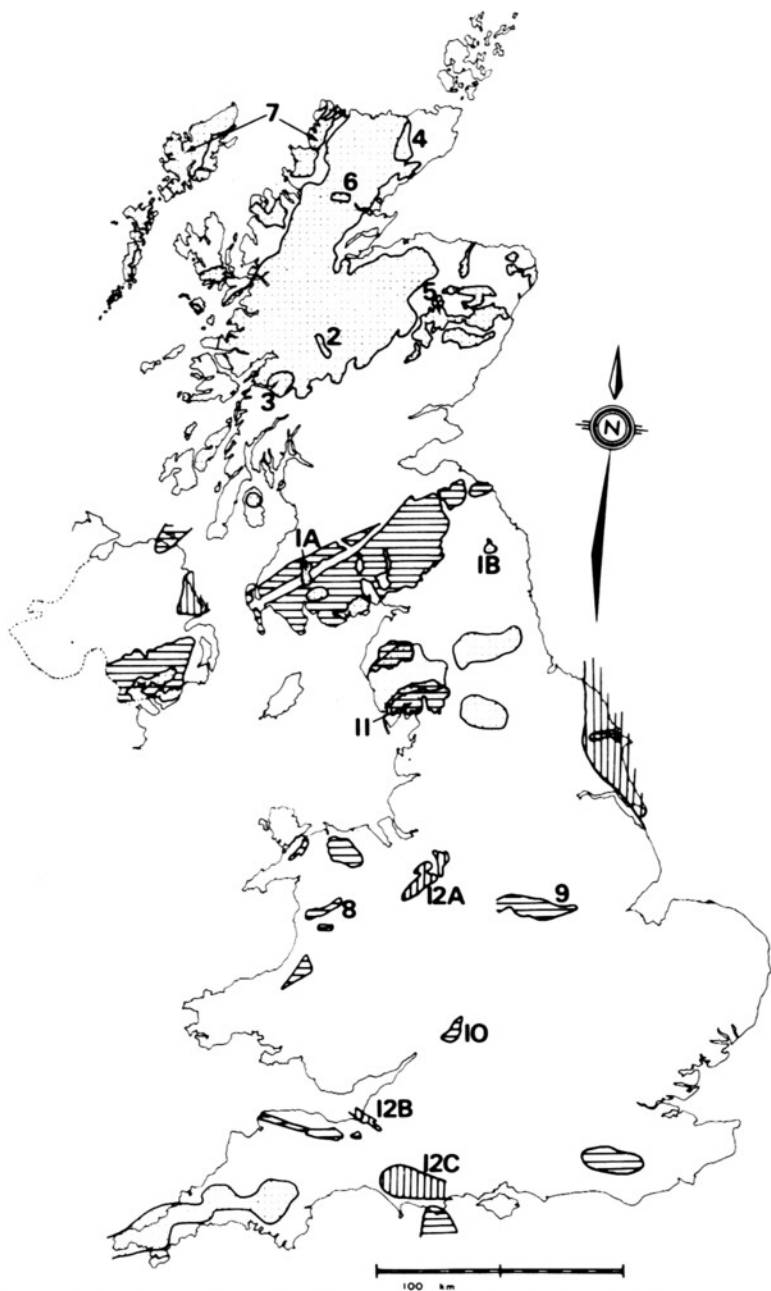
Map showing the distribution of rocks thought to meet the selection criteria and of those areas which have been selected for feasibility studies. Crystalline igneous and metamorphic rocks are stippled, argillaceous rocks are shown with horizontal lines and evaporites with vertical lines. The crystalline rocks include the postulated subsurface outcrops of the granites of northern and south-western England. No rock types meeting the criteria occur in the Shetland Islands.
