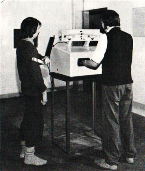
Personnel working in active areas of buildings monitor their hands, clothing and shoes before leaving.
