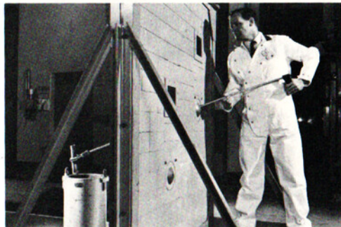
Here, a mobile lead wall is used for handling a source giving rise to high level beta gamma radiation.
