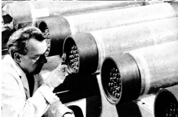
Advanced Gas-cooled Reactor fuel assemblies.
