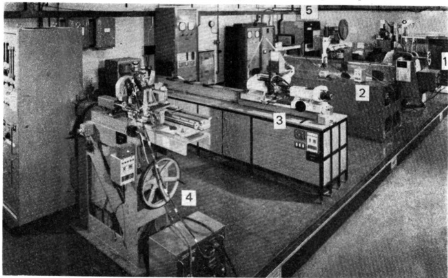
Fig. 1. General view of welding equipment showing 1. Tube to tube-plate welding gun mounted on manipulator 2. X Y Z manipulator 3. Butt welder 4. General purpose manipulator 5. Computer-based control unit.
