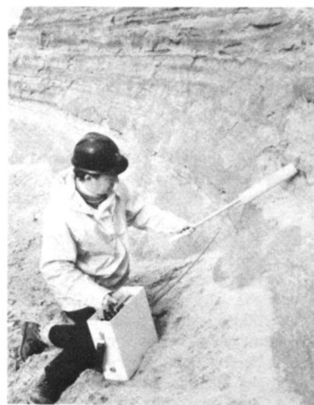
This 4-channel gamma spectrometer developed by Harwell measures simultaneously uranium, thorium and potassium concentrations
