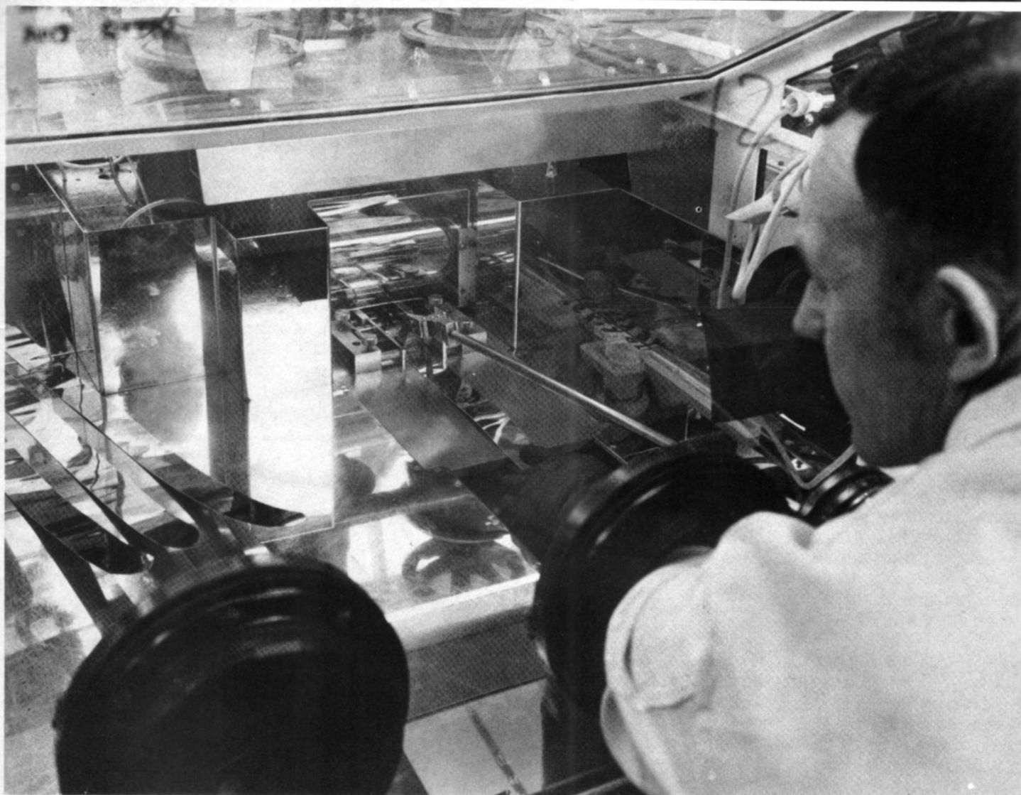
A close-up of glove-box work in foil manufacture at TRC.
